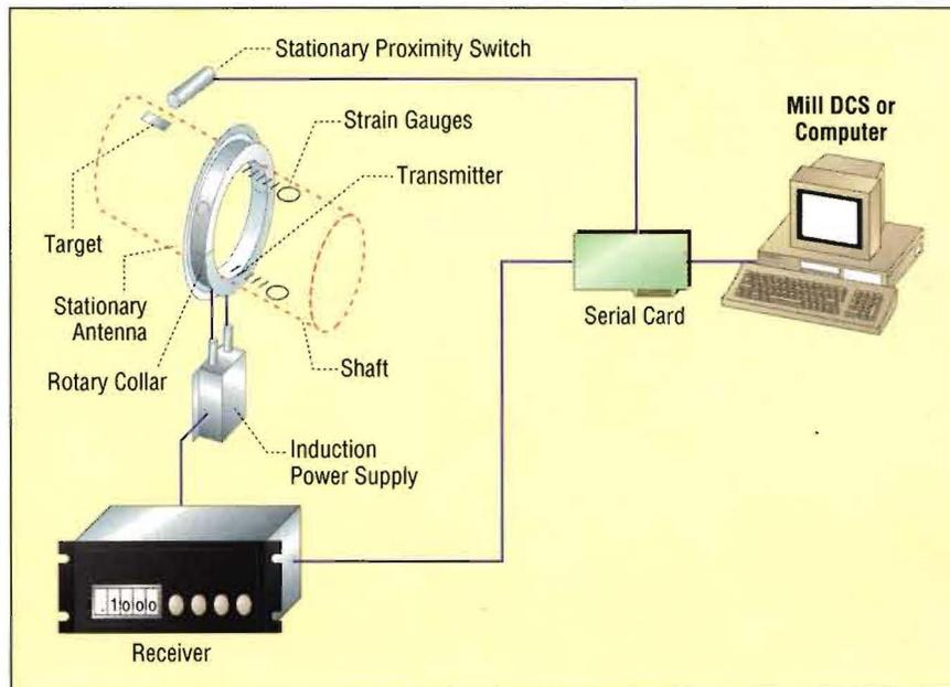
Taking advantage of the engineering relationships between torque and stress, as well as stress and strain, the software performs the calculations to display the transmitted torque in numerical or graph form. Shaft RPM is also measured and displayed and, from shaft RPM and torque, the horsepower can be calculated and graphed.
