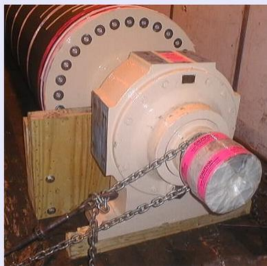
To avoid the risk of damage, whenever possible, the bearing housings and bearings should be removed from a roll prior to transportation. If not possible, the roll and bearing housing should both be blocked in a way to support both the roll and bearing housing to reduce the stress load and vibration transmission into the bearing.
