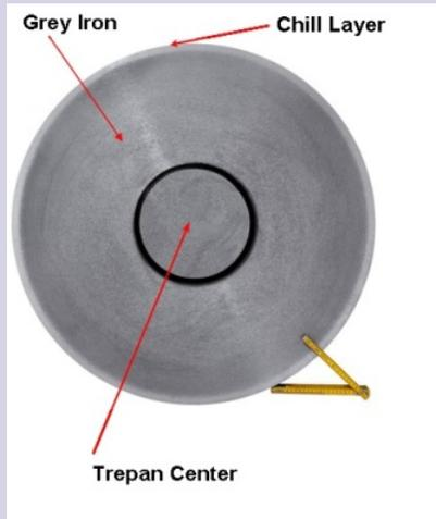
The chilled iron is significantly harder than steel and non-chilled iron. And it is this hardness that is desirable in calendar rolls as it improves the roll's ability to maintain a good profile for a longer period of time.
